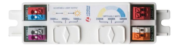
With the switchable option, a single module allows you to easily select between 3 color temps and 3 lumen outputs - 9 SKUs in 1 strip!
